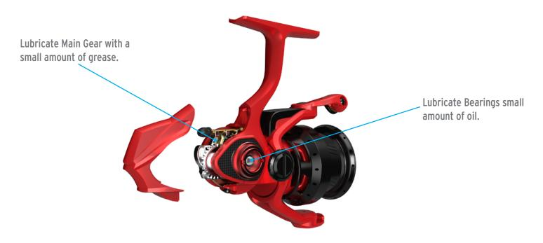
To keep your reel working at peak efficiency, clean and lubricate after each use. At least once a season your reel should be disassembled for a thorough cleaning and re-lubrication. Refer to the exploded parts view supplied with your reel. Reel maintenance kits can be purchased at your local tackle store and include everything you need to properly service your reel. If you do not wish to perform this work yourself any nearby Abu Garcia® Service Center is fully qualified to do this for you.
